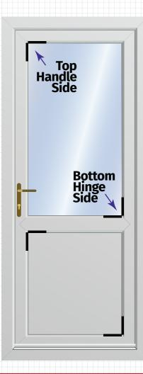
When installing glass or panel into a uPVC or Aluminium Door, it is essential that the glazing is "toe and heeled".
