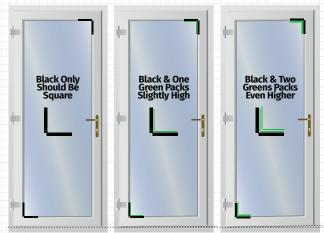
WE WOULD ALWAYS RECOMMEND ENSURING THAT THE FRAME IS SQUARE & GLASS IS TOE AND HEELED CORRECTLY BEFORE ADJUSTING HINGES
